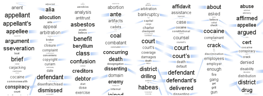
FIGURE C.11: Edge stubs are drawn in a single hue. Complete edges are only shown on hover or select. Advantages: edges do not interfere with legibility, stub direction indicates destination, stub shape indicates relative size of words on each end of edge, simple colouring creates a pleasing aesthetic. Problems: without hover or select, determining the destination column for a stub is not possible. This is the version used in the final prototype presented in Chapter 6.
