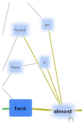
FIGURE 4.7: Edges connecting a node are highlighted on mouse over to clarify edge crossings.
